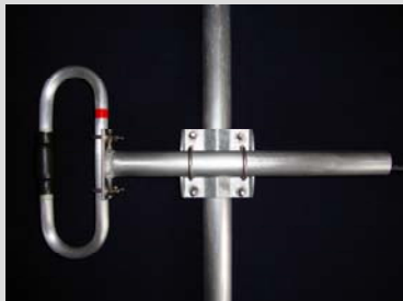
1/4 - wave spacing (3.5 - 4.2 dBd gain) (Offset pattern)
