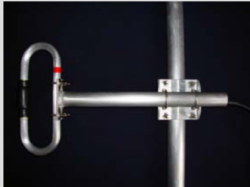
1/2 - wave spacing (8 dBd gain) (Bi-directional / Elliptical pattern)
