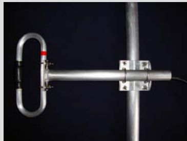
1/2 - wave spacing (3 - 3.7 dBd gain) (Bi-directional / Elliptical pattern)
